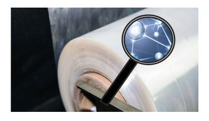
So, how exactly does this happen? The science of shrink wrap can be explained in terms of molecular behavior. The molecules of a shrink film sheet or tube are randomly intertwined,
